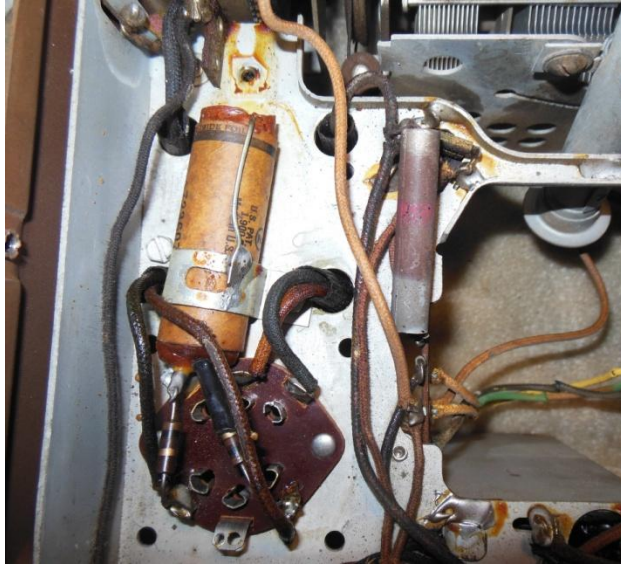
Left: old dual buffer capacitor
