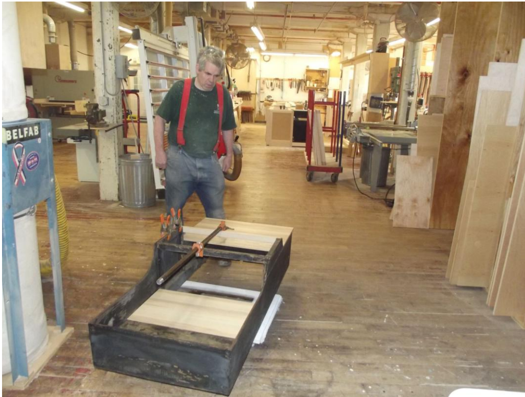
Body with new ash parts installed
