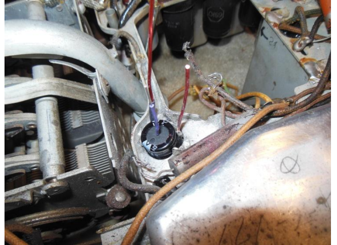
Dual electrolytic (middle, 3 wires) being replaced; tuner and pushbutton clutch to left
