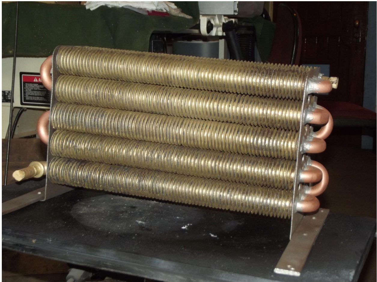
Brass and Copper Radiator after glass blasting
