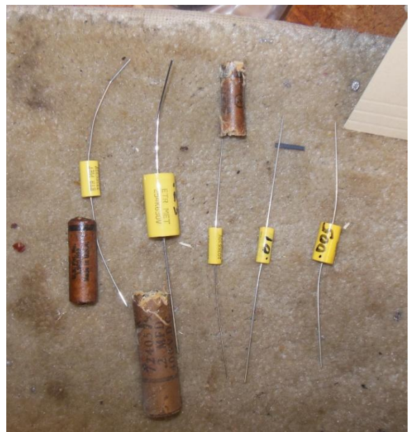
Old paper (wax) capacitors and new polypropylene replacements
