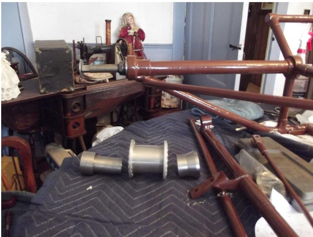
**Photo 2: Construction of steel core to fit rear hubs**
