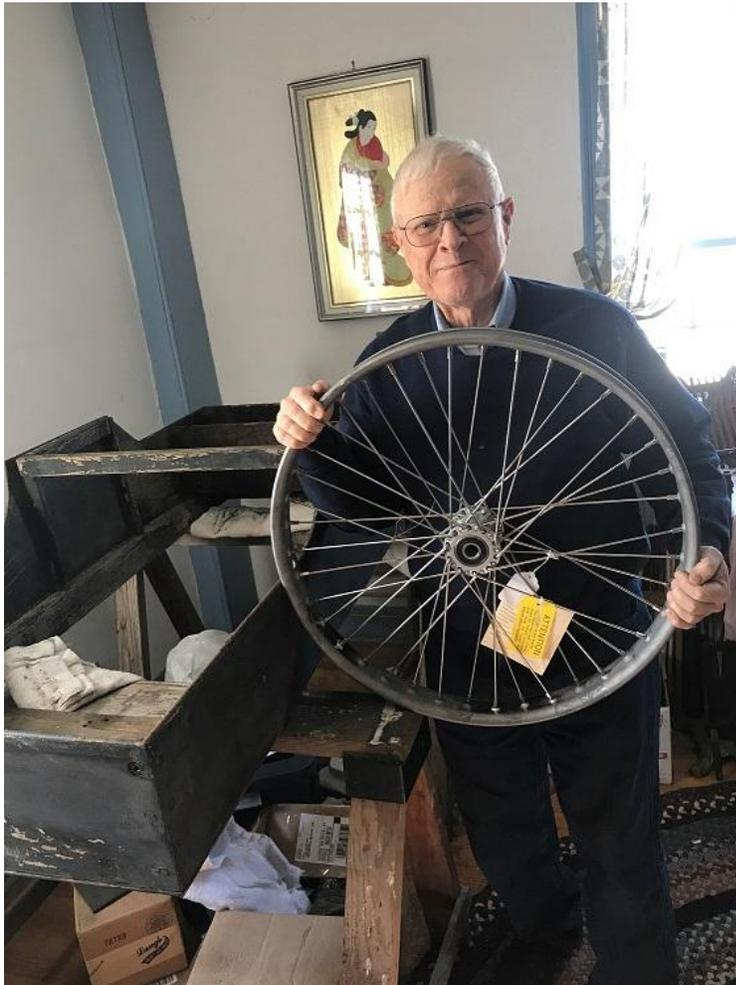
I shipped the hubs and rims to Buchanan Wheels in California. They are a well-known constructor of wire wheels for motorcycles and now for Orient runabouts. They did a wonderful job of fitting each rim with 40 dimples, about the size of your thumb, to hold the 40 new spokes between the rim and the hub. (photo 3)
