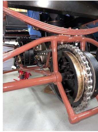
In the next photo Charlie and I are removing the small sprocket for the transmission drum. Charlie would machine the face of this sprocket to make it fit closer to the drum. The reason that the chain did not fit properly on the sprockets is because the rollers are .625 in OD. We have determined that the proper size is .5625. Charlie made
