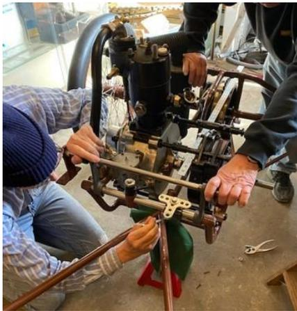
In the photo to the left you can also see a three foot aluminum measuring tool. This tool is lying against the points on the sprocket to check our alignment changes.
