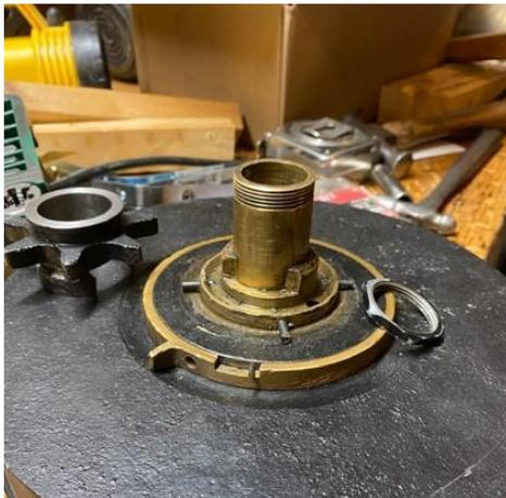
shaft firmly holds the sprocket which is press fit into the bottom of the shaft hub. It turns in whatever direction the bronze plate is moved by the gears. The sprocket then moves the differential which
