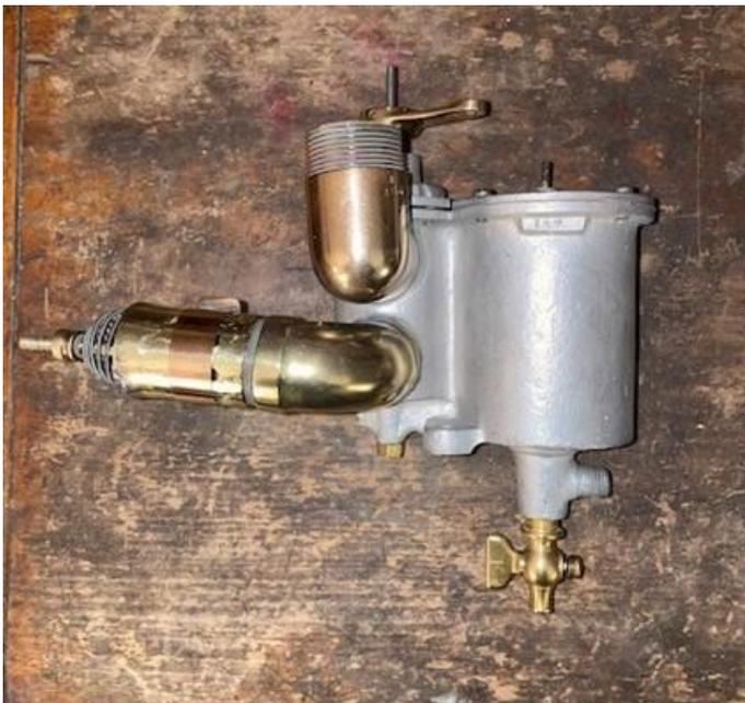
The lower elbow on the carb in this photo has a valve in the cylinder that controls the air as it enter the carb. It is a leather valve that is held close with a light spring that is similar that on the intake valve. This valve opens when the engine is on the intake stroke and is sealed on the other three stroke.
