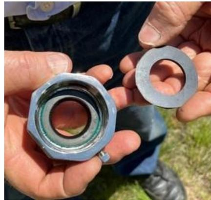
We also had experienced a oil leak on the transmission shaft. I mounted two seals inside of the packing nut the Frank made for the engine. The shaft seal is located inside the packing nut and the seal of the outside diameter of the shaft bearing is slid over the shaft and held in place with the threaded nut.
