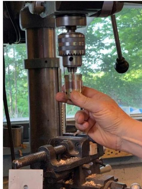
I have made a neoprene disk that will be the new seal in the carb. I will replace the leather seal with a fender washer to provide support for the neoprene.
