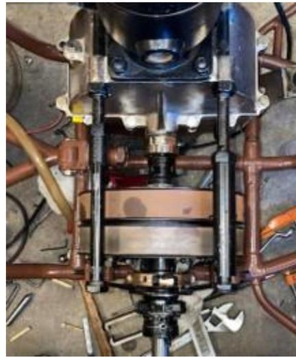
For the third test of the engine, I assembled the transmission onto the shaft. The next step to prepare of our next run was to figure out how the muffler was mounted and secured to the engine. Since the muffler was not on the car when I bought it I did not know exactly where it went but I did figure it out.
