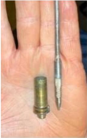
could not do last time. There are now new improvements that we need to make. The first is the sensitivity of the air-fuel adjustment valve. In the photo to the left, you can see the needle and the seat. On this original design the needle tip is screwed into the seat. You can see two of the three parts of the
