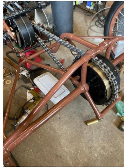
In addition to the chain, we needed to do some work on the sprockets to make the chain straight when it is in the car. Charlie did this by facing the sprocket and the packing nut that is on the crank case. We then mounted it all and I think it looks excellent.
