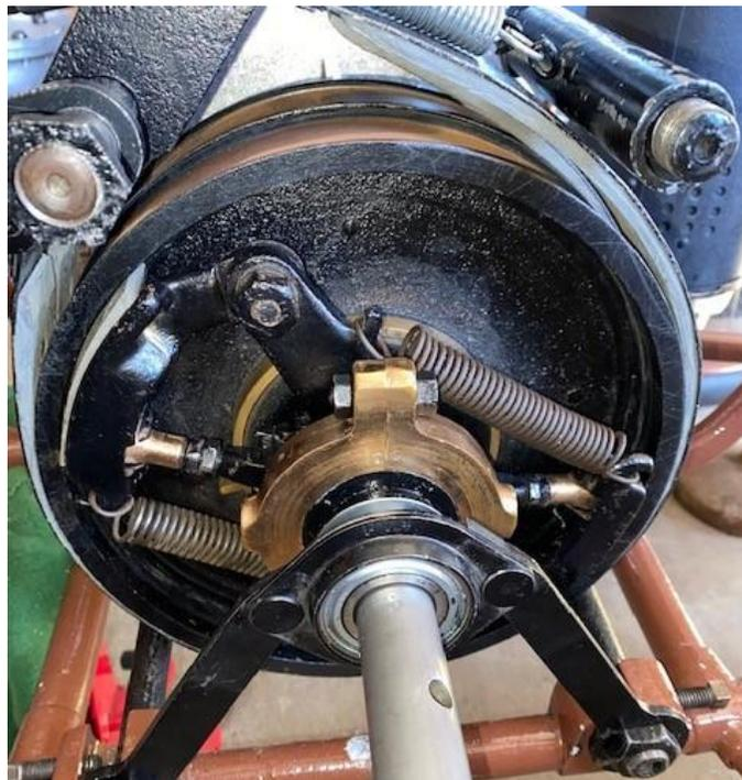
The next thing that we began work on is the clutch. This photo shows the clutch which is located on the inside of the nearest transmission drum. As you try to figure this part out, realize that the function of the clutch is very different on this car as compared to modern ones. In a modern car, you select the gear you want by holding the clutch in and then let the clutch up to engage the engine to the transmission. On the 1901 Orient, the only engagement of the clutch is for high speed.
