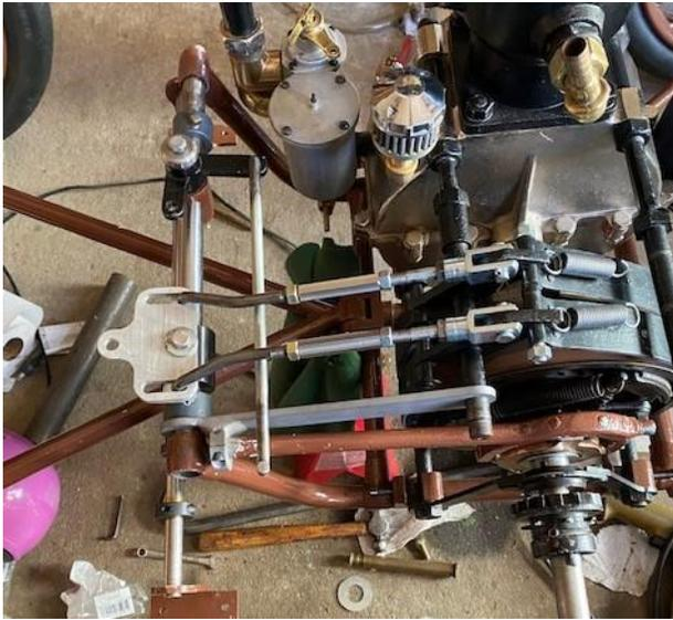
The pedal is attached to a black "L" shaped piece which is mounted to a pivot point on the cross chassis rod. A rod connects the "L" to the pedal and another rod connects it to the clutch control rod.
