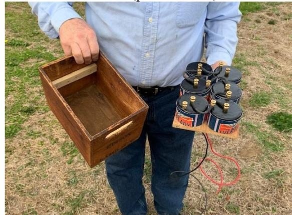
I have fabricated false dry cell tops and installed them on a wooden panel inserted in the Edison box that holds them. Under this wooden separator, I will install a motorcycle battery to provide the car with the necessary electricity.
