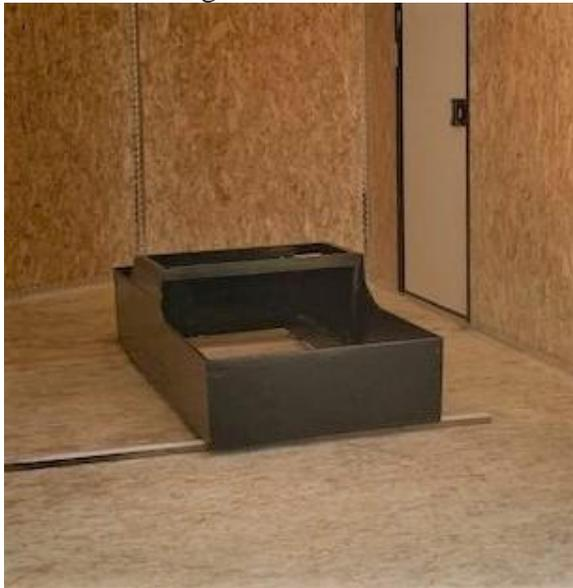
I am brush painting the 119 year old body using that same procedure that was originally utilized when it was first constructed. I will apply a final coat (in the warm weather) before I assemble the chassis and metal parts over the wood.
