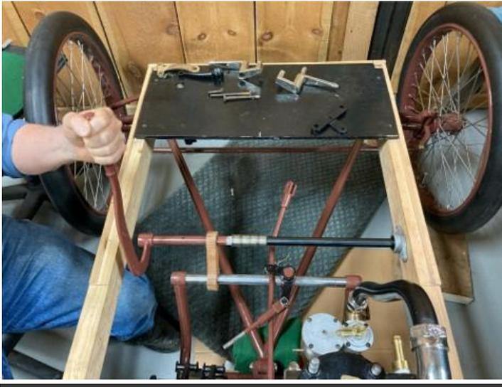
The lever that I have in my hand is a part that came with the car. It is quite a bit smaller than the lever used in 1902. I am working on a location that keeps the original steering column and body. I have extended the shaft for the rod to the sill of the car. The left can be supported by a connector that is shown as wood in this photo.
