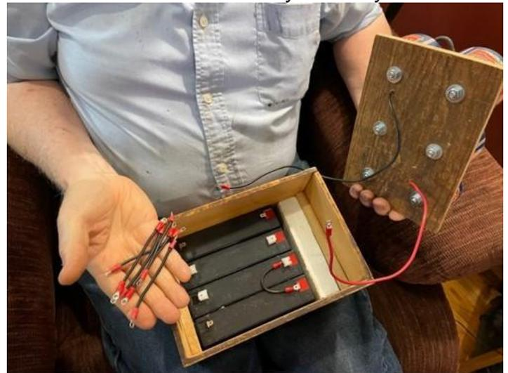
These are six volts and will be wired in parallel. This should allow me to run the car for one day.
